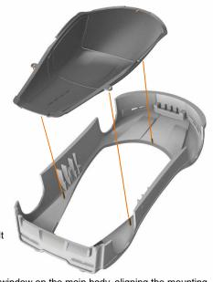
Position the Lexan window on the main body, aligning the mounting tabs with the guide pins. Secure the Lexan window to the body by melting the guide pins with a soldering iron or put CA glue.
