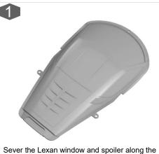
designated cutting line. Then, drill a small hole in each of the three mounting tabs.
