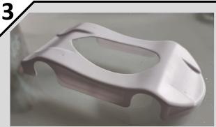
Using a DREMEL-type tool to remove the remaining plastic until the marker line disappears.
