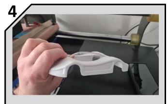
Glue the lexan roof with LOCTITE or EPOXY type glue, taking care to lightly sand the contact areas.
