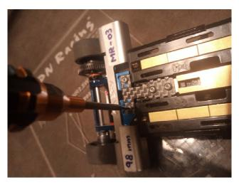
Tighten the T-Plate screws correctly, it is possible to remove the Brick Pod, and you can verify that you have found the starting setup in an instant.
